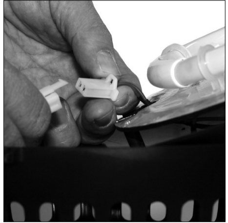
Disconnect the wires (fan and switch connector).
